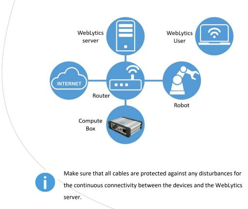
The illustration above shows the recommended network configuration. It is possible to deploy WebLytics in a different configuration, e.g., with several IP subnetworks connected by one or more routers. Regardless of the specific network configuration, it is important to ensure that the WebLytics requirements are met, to ensure a successful WebLytics installation and operation.
