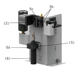
1.4 Manually push up the cleaner motor until the reamer enters the welding gun nozzle. The gap between the reamer and the welding gun nozzle is identical around the circumference. If necessary, adjust the position of the welding torch.
