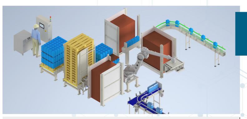
The robot cell provides the ability for manufacturers to create palletized bottled water stacks, ready for shipping. The two incoming conveyors allow diversifying the stacked bottle types. This system has been designed to accommodate **5L plastic bottles as well as 3 x 2L bottle sets.**
