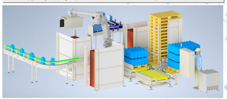
The core strength of the cell is the **rotating conveyor technology** that allows us to create a very compact system while still retaining high functionality and versatility.
