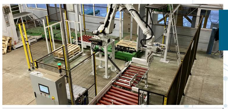
The automated cell palletizes peat bags into multi-layered, transport-ready stacks. The system gives the enduser a wide variety of functionality with customizable parameters, while retaining all the benefits of an easy-touse, compact system. The cell consists of two incoming peat bag-positioning conveyors, pallet stock, a placement tower, a human-machine interface screen, a robot, and its claw, and a mounting platform, as well as its controller.
