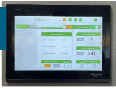
Using the HMI screen, cell operators can not only monitor the current state of the cell, but also create multiple peat bag orientation and offset configurations and then save them in the system's database. The screen provides additional functionality such as manual control of the cell and work mode selection.
